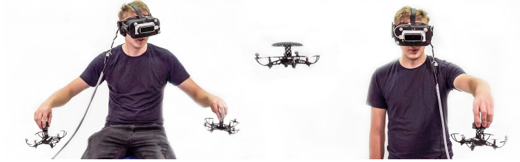
Figure 4.1: Left: A user piloting an aircraft in VR. The user has a slider in his right hand to control the speed. With the joystick in his left hand, the aircraft can be steered sideways. Right: A user is rotating an object in VR using a knob.
