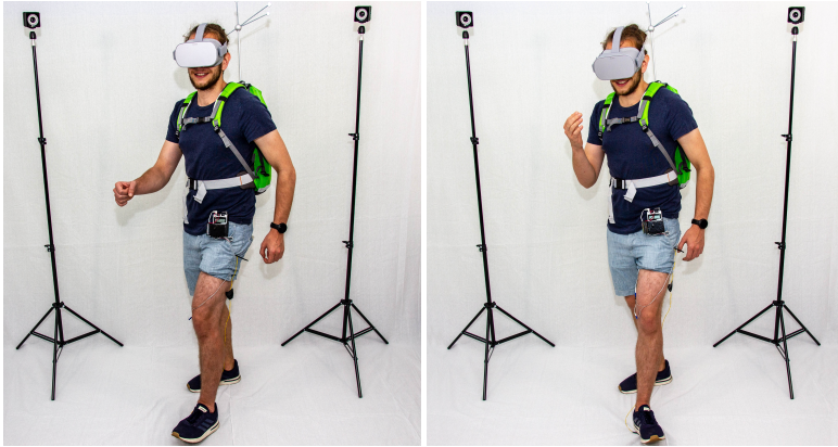
Figure 6.1: Left, the user walking in VR on a straight path. Right, the user's leg is rotated via EMS to the left. Through this actuation, the user walks in a circle (staged scene).
