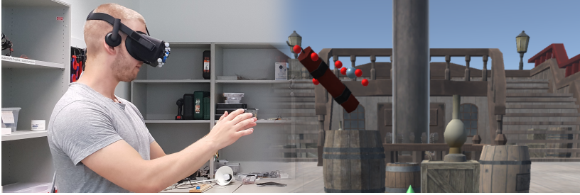
Figure 3.1: A VR user interacting with a stick of dynamite. The physical counterpart of the virtual dynamite is optically tracked in real-time through VinteR . Through that, the user is capable of catching the dynamite.
