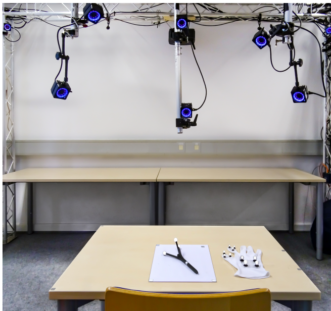
Figure 8.3: Hardware setup of the VRSketch system where hand, pen, paper, table, and chair are tracked via configurations of retro-reflective markers. Seven of the eleven OptiTrack cameras are close to the table for more precise tracking.
